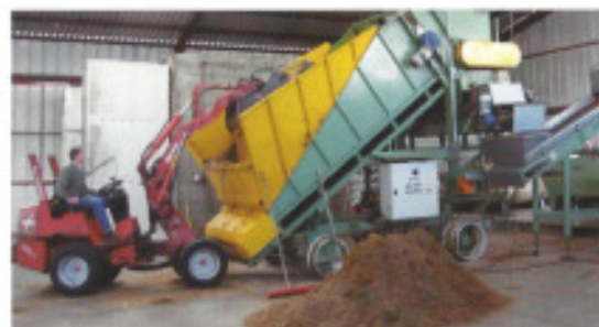
Filling and inoculation line for shiitake substrate.
